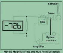
Both MK1 and the AUTO work on the basis of stationary sample and moving magnets. Two pairs of magnets are placed at opposite ends of a beam making a balanced system having a magnetic field at each end. Introduction of the sample into the magnetic field attempts to deflect the beam and the
